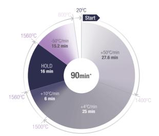
The sintering recommendation is only a guideline; some adjustments may be required depending on each individual furnace. If the furnace cannot be set according to the 54- or 90-minute sintering schedule, speed sintering cannot be used.
