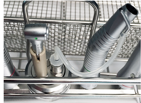
Connection example, adapter for external spray channels
