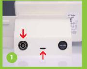
Connect the basic unit to the power supply ( $\downarrow$ ). Check whether the SD card is placed in the SD card slot ( $\uparrow$ ) in the back of the basic unit.
