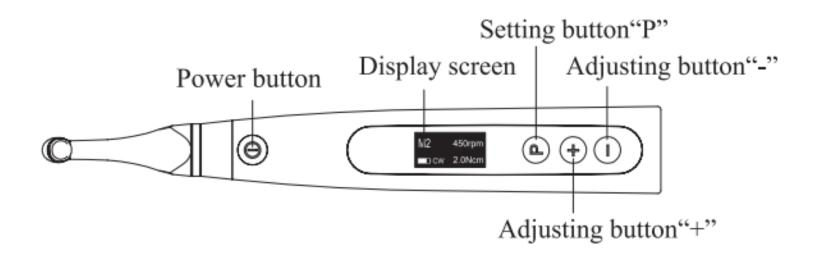
To power ON the device, press the Power button.
