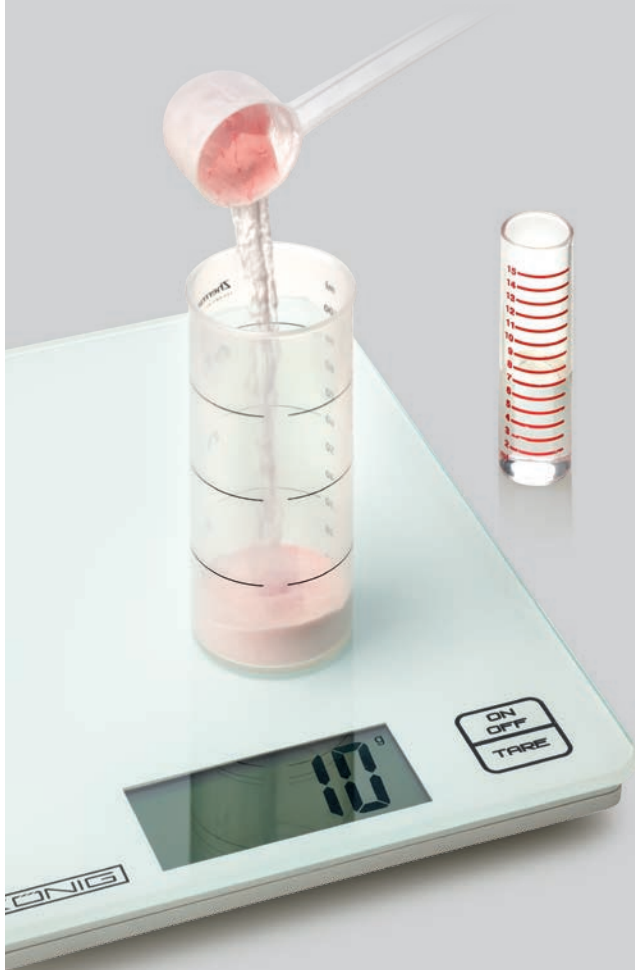
Weigh the resin, measure the monomer and mix, pouring the monomer in first and then the resin
